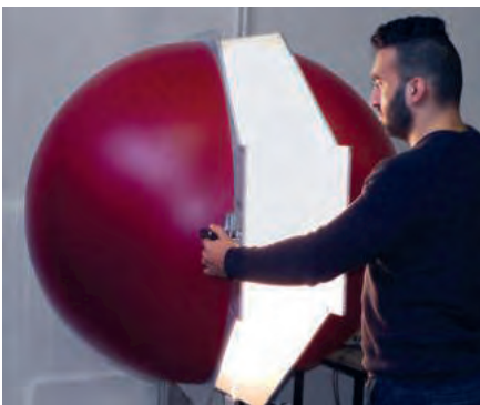
We use the Ulbricht sphere for the measurement of the luminous flux of luminaires in our lighting laboratory.
